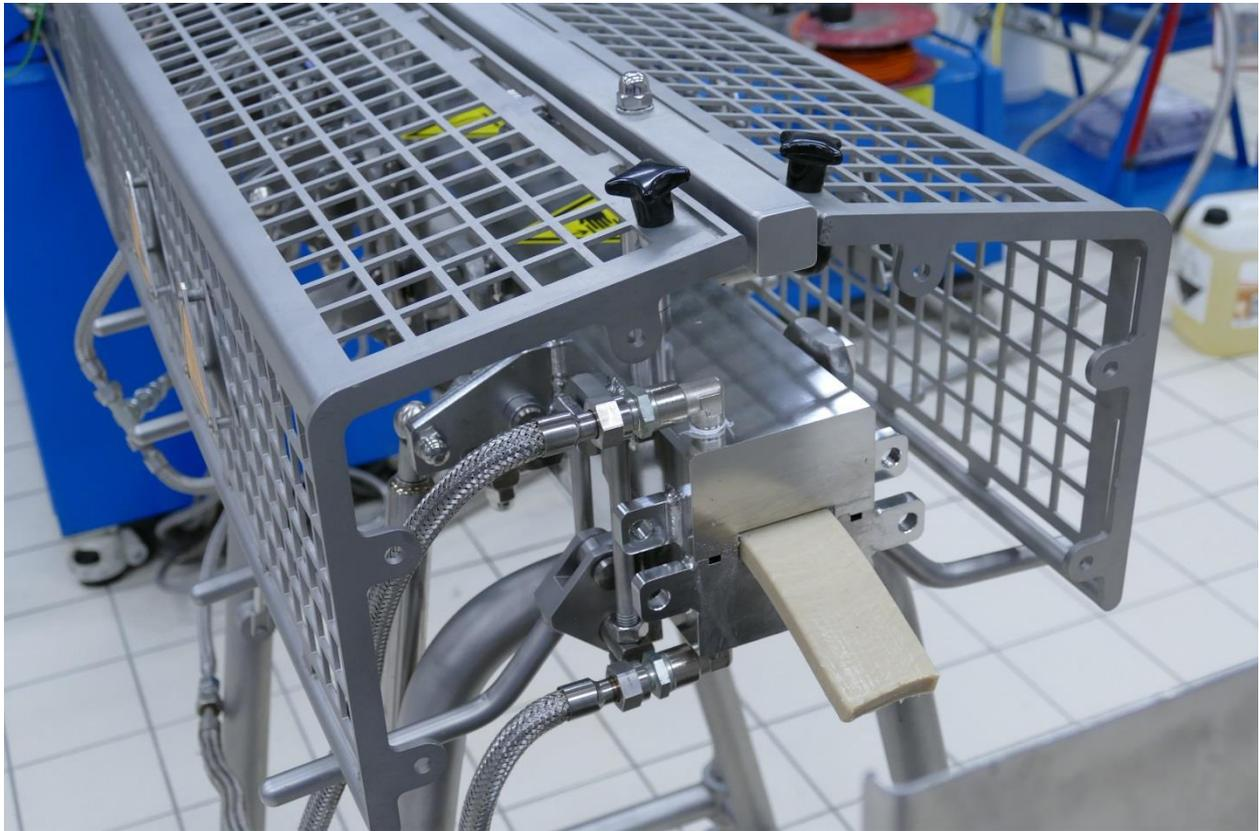
High Moisture Meat Analogue (HMMA) discharging from the cooling die flanged directly to the Coperion ZSK food extruder.
