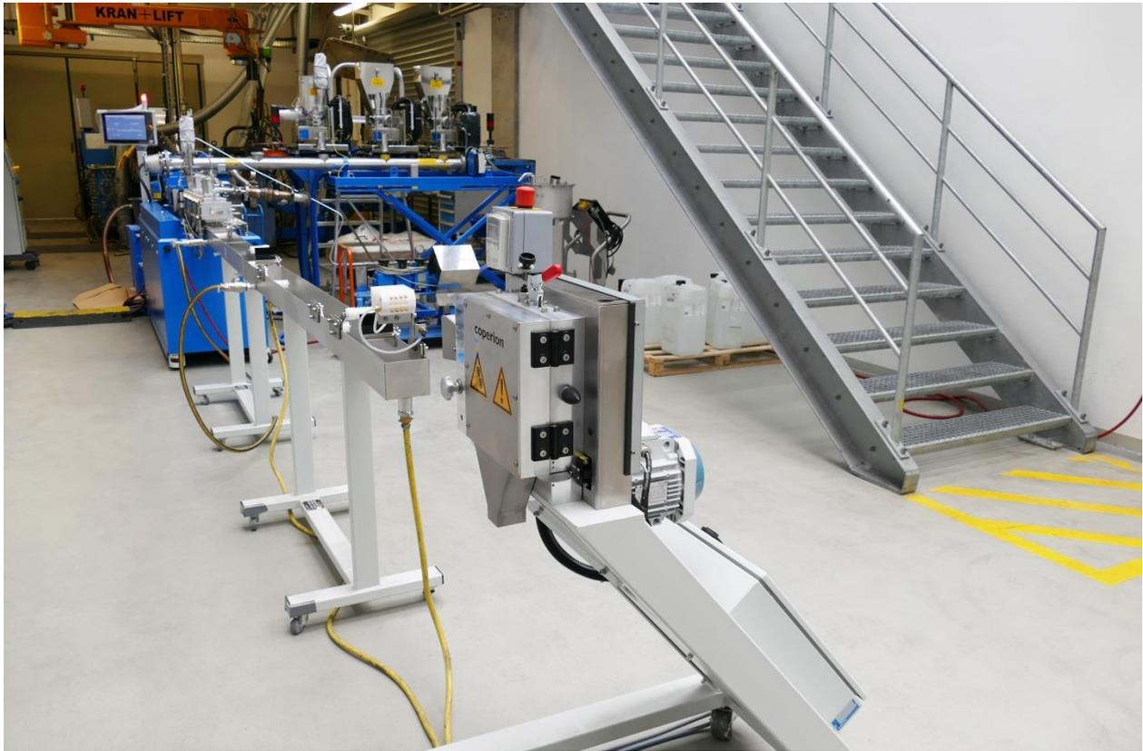
*Complete lab-scale system for Asahel Benin Sarl., consisting of a ZSK 26 Mc<sup>18</sup> twin screw extruder, four feeders from Coperion K-Tron, as well as a water bath, air wipe and SP 50 strand pelletizer from Coperion Pelletizing Technology.*
