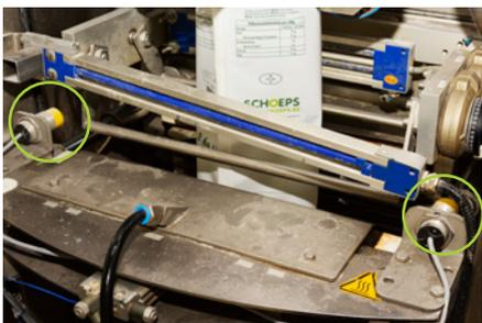
Sensors are mounted to the sealing bars of the packaging machine
