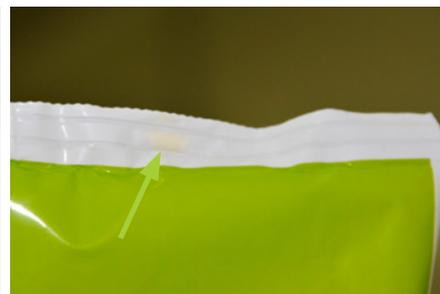
Cheese parts in the seal in a bag rejected by **SealScope™**
