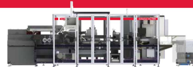
The CLI-CMI Series cartoner is for packaging lines that want maximum flexibility with low to medium speed capabilities. This machine has a compact footprint to fit tight spaces on your packaging floor. Flexibility is provided by quick changeovers and the largest carton size range in the industry. The optional IndeCart® 3 bucket transport enhances the flexibility by de-coupling the upstream process from carton loading.
