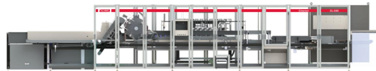
The CL-CM Series cartoner is for packaging lines that want to maximize throughput, with some of the fastest speed capabilities in the industry. Large pitch and medium pitch versions are available to meet your production needs. Flexibility is provided by quick changeovers and a capability to run a large range of carton sizes. Standard configurations are available to provide the best performance and highest speeds for bag-in-box products.
