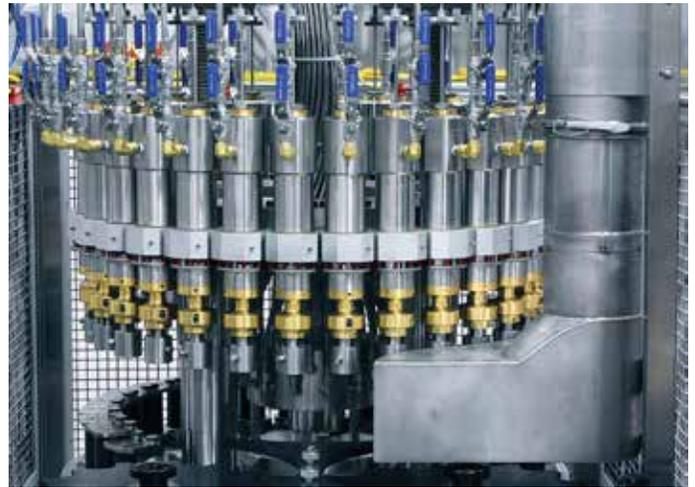
Through-The-Valve (TTV) Propellant Filler
