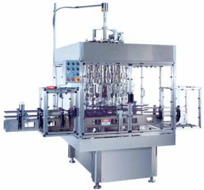
KP-Aerofill AG-275 is available in 12- and 18-head configurations. The heavy-duty base construction provides a rugged foundation which helps minimize vibration and noise levels, even at maximum output. The 5 hp explosion-proof-rated, variable frequency drive controls machine rotational speed, delivering up to 17 RPM.
