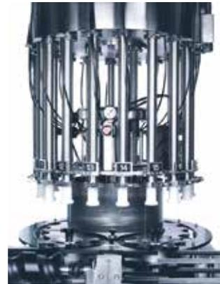
The C.I.P. Rotary KP-Aerofill AE-600 meets all 3-A Sanitary Administrative Council standards for cleanliness and bacterial control. The Electronic No-Container No-Fill (ENCNF) System detects the presence of a container for each head. If a container is not present, the system prevents the dispensing of product eliminating waste and reducing costs.
