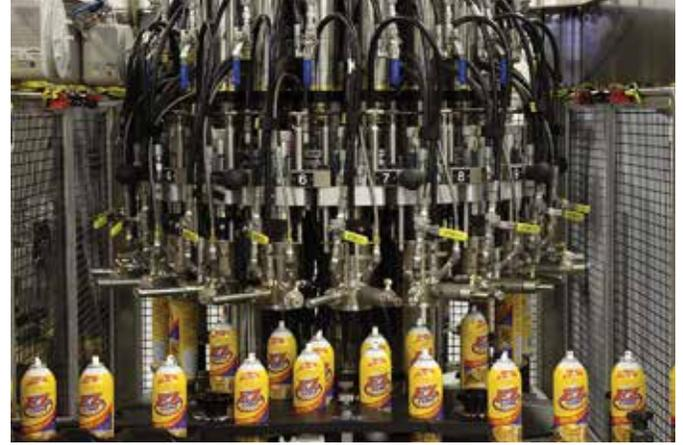
Rotary Under-The-Cup (UTC) Propellant Filler
