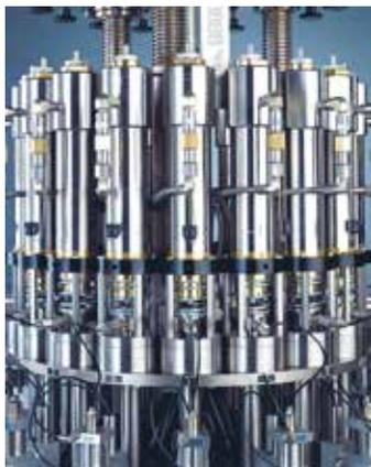
Positive displacement propellant powered metering cylinders ensure precision fills. Cylinders have a capacity of 550cc and are propellant powered eliminating heat buildup typical with air powered cylinders when using compressed gasses such as CO<sub>2</sub> and N<sub>2</sub>O. KP-Aerofill AG-275 offers 249 degrees of rotation for propellant filling and 226 degrees of rotation for shaking.
