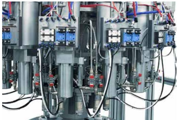
Through-The-Valve (TTV) Air-Powered Propellant Filler
