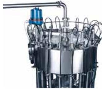
Standard level controls are replaced with simplified electronic level controlling device.
