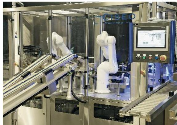
With a cycle rate of 600 units per minute, two Stäubli six-axis robots perform the process of separating empty and grouping filled glass containers.
