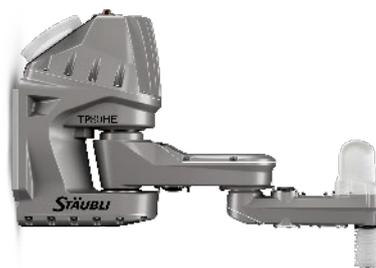
FAST picker TP80 for humid environment (HE), is lubricated with food grade NSF H1 oil without any loss of performance.
