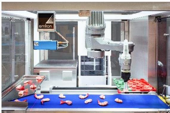
Our FAST picker TP80 HE is the only available clean picker worldwide. This high speed packaging cell is equipped with 3D robot guidance.
