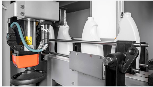
Bottle Orientation for asymmetric bottles for specific alignments
